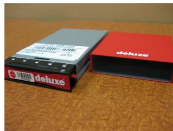
CRU with casing removed
