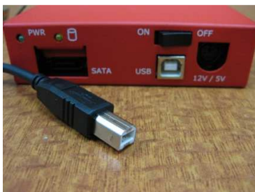
CRU standard USB-B connection
